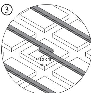
If the head ends of the floor joists are placed against each other, provide an overlap of at least 10 cm. (fig.3).
