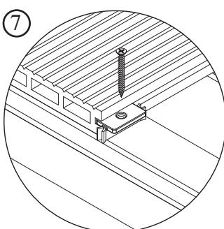
When two decking boards are placed together with an installation clip, screw the clips in the floor joist ( fig.7).
